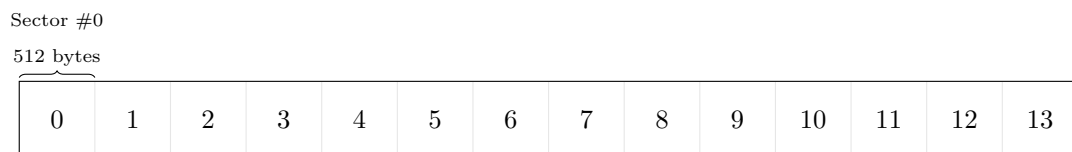
Figure 2.1: A block device with 14 sectors and 14 \times 512 = 7168 bytes total
