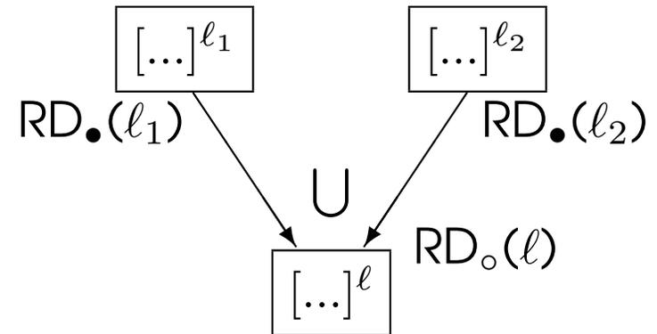
$$RD_o(l) = \begin{cases} \{(x, ?) \mid x \in FV(S_{\star})\} & : \text{ if } l = \text{init}(S_{\star}) \\ \cup \{RD_{\bullet}(l') \mid (l', l) \in \text{flow}(S_{\star})\} & : \text{ otherwise} \end{cases}$$
