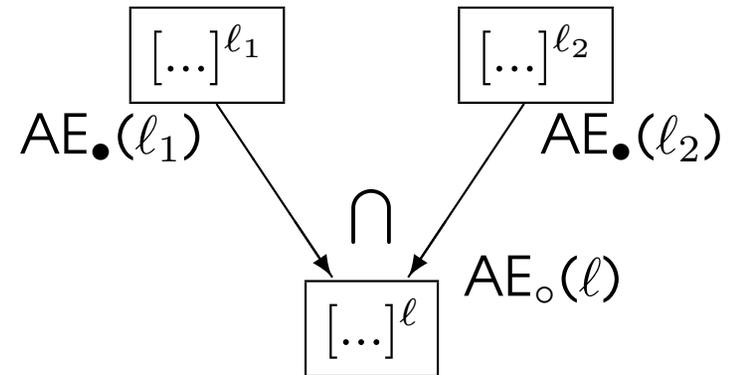
$$AE_o(l) = \begin{cases} \emptyset & : \text{ if } l = \text{init}(S_\star) \\ \bigcap \{AE_\bullet(l') \mid (l', l) \in \text{flow}(S_\star)\} & : \text{ otherwise} \end{cases}$$
