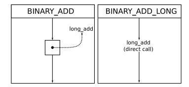
Replacing the indirect call with a direct call.
