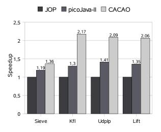
Figure 3: Performance of picoJava-II and CACAO/YARI for some embedded benchmarks, normalized to JOP.
