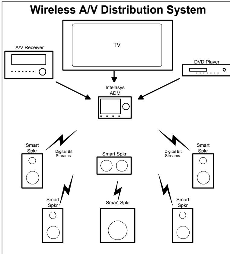
identified themselves as left and right and are extracting the audio stream for the left and right respectively. The operator could push a button on the A/V receiver and switch left and right without moving or reconnecting any cables.
