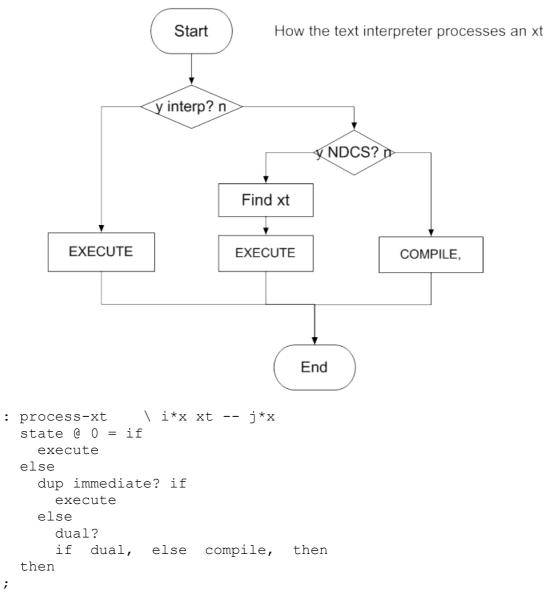
The picture illustrates a Forth interpreter/compiler loop that has been modified to cope with separated interpretation and compilation actions.
