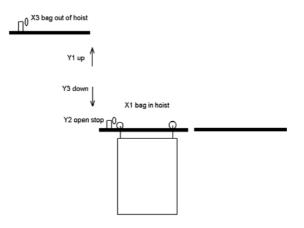
A container runs by gravity into a vertical conveyor, is elevated, and runs off to a storage position.
