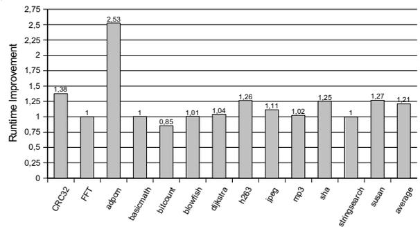
Fig. 7. Speedup in comparison to the existing compiler based on gcc.
