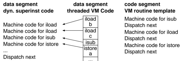
**Figure 2.** A dynamic superinstruction for a simple JVM sequence
