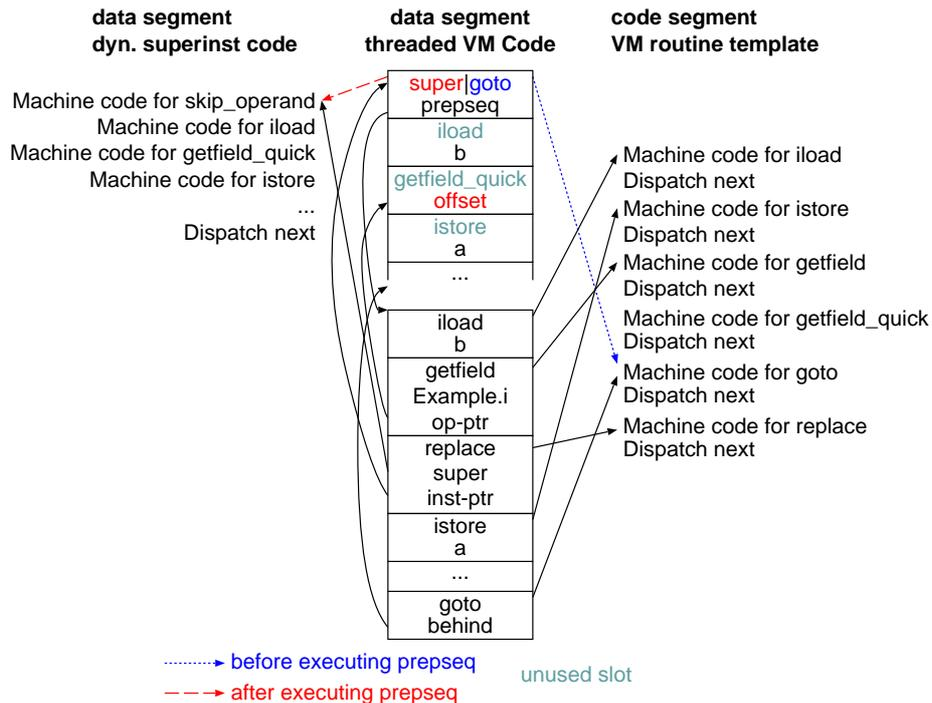
**Figure 5.** SableVM’s preparation sequence for the first execution and the dynamic superinstruction including a quick instruction for subsequent executions
